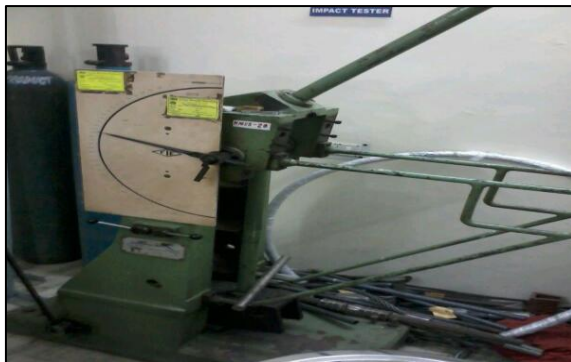
Fig 2: RESULT: The Impact Value for the Axle Shaft Was 124 Joules.
